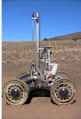
RESOLVE drill on Scarab rover
