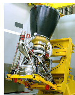
An RS-68A being prepared for installation on a Delta IV CBC (Aerojet Rocketdyne)
