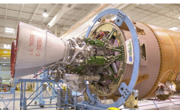
An RD-180 engine installed on the first stage of an Atlas V (ULA)
