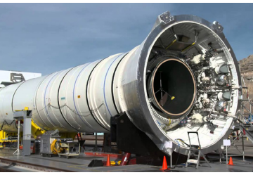
A 5-segment Solid Rocket Booster being prepared for ground test firing (Orbital ATK)
