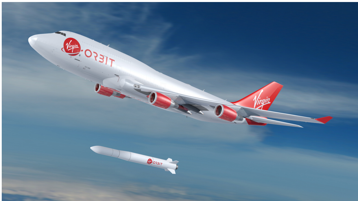
An artist's impression of the LauncherOne vehicle integrated with a Boeing 747-400 carrier aircraft. (Source: Virgin Orbit)
