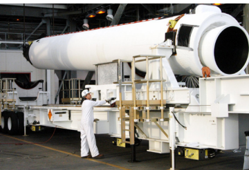
A GEM-60 being prepared for integration on a Delta IV (Orbital ATK)
