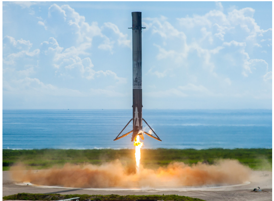
A Falcon 9 first stage returns to Cape Canaveral Air Force Station during a mission conducted in 2017. (Source: SpaceX)
