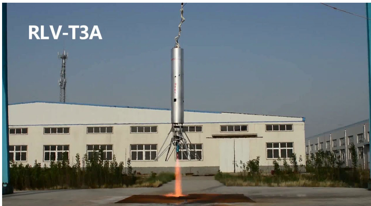
Link Space conducts a hover test in 2016 using a tethered testbed vehicle. (Source: Link Space)
